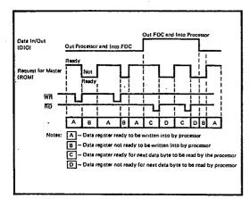
Figure 3. Status Register Timing
